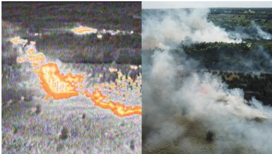
Figure 14. The fire event viewed with two different cameras, conventional RGB (right) and infrared (left); Source: ( https://extension.okstate.edu/fact-sheets/using-drones-with-infrared-capabilities-to-monitor-fire-behavior.html )
